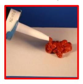
FlameShield™ fire rated acrylic intumescent caulk is designed to prevent the spread of fire from one compartment to another wherever services wires, cables and pipes penetrate separating walls and floors, or wherever a gap remains between elements in fire rated walls or floors.
