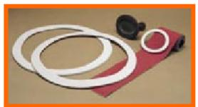
These gaskets are made from TFF universal fabric and is especially suited where a rough or uneven surface or flange exists. The fabric is a fiberglass base with a special white rubber formulation. The fabric is tacky, and has a plastic film surface covering that is removed before installation. The fabric will stick to itself once the film is removed.
