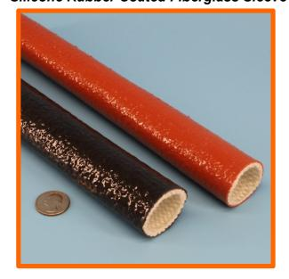
FlameShield<sup>™</sup> Marine grade firesleeve allows properly assembled hose assemblies to meet ISO 15540 testing. We also maintain traceability records for customers buying this product. 500°F / 260°C continuous rating and with a 30 minute "Fireproof" 800°F / 426°C rating. Also meets 14 CFR 25.869(a)(4); Appendix F, Part 1(b)(7) (60-degree flammability Test) for use as a wiring/cable protection sleeve.
