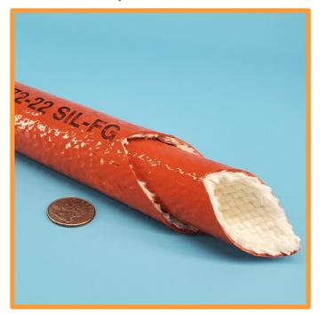
DualShield<sup>™</sup> firesleeve is built from two layers of aviation grade sleeve, providing superior protection to hoses, wiring, cables and tubing from heat, flame, molten splatter, sparks and other environmental factors. The first completed sleeve is oversleeved with another layer of fiberglass braid, and that braid is also coated with the same thick coating of self-extinguishing silicone rubber.
