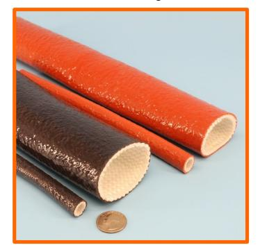
FlameShield<sup>™</sup> MSHA Mining approved firesleeve protects hoses and lines on mobile and fixed mining equipment. 500°F / 260°C continuous rating and with a 30 minute 800°F / 426°C rating. Also meets 14 CFR 25.869(a)(4); Appendix F, Part 1(b)(7) (60-degree flammability Test) for use as a wiring/cable protection sleeve.
