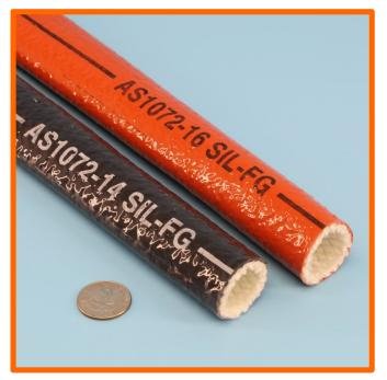
Hytec-Bosch-Rexroth FS series Aviation / Aerospace grade equivalent firesleeve is manufactured to the SAE AS1072 specification. CofC and Test Report available with orders. Our company QMS has been reviewed and accepted by major aerospace OEMs. Allows properly assembled hose assemblies to meet SAE AS1055D testing. 500°F / 260°C continuous rating and with a 15 minute FAA "Fireproof" rating when assembled according to SAE AS1055. Also used for Heavy Duty Industrial hydraulics applications.
