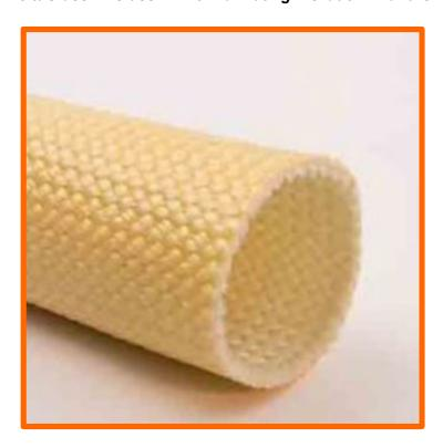
This high temperature and heat resistant braided hermetic fiberglass (fibreglass / glassfibre) sleeve, fabricated from high quality E-Type fiberglass filaments that will not burn and has been saturated with a high-crosslinked modified acrylic copolymer.
