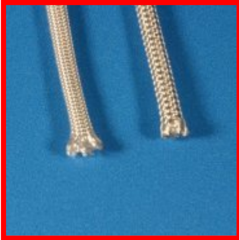
S-Fiberglass Sleeve: Plain & Heat Treated
