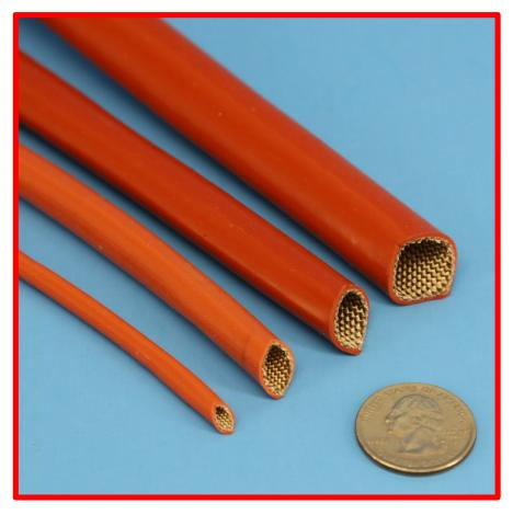
FlameShield<sup>™</sup> small diameter firesleeve with Heavy Wall Silicone Rubber coating is designed as a primary insulation sleeve for protecting small diameter wire, cable, lines, hose, and pipe from high temperature, flame and environmental contamination. Recognized by UL / CSA for 240°C, 600V service, and meets VW-1 flammability requirements.
