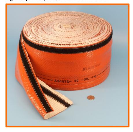
ZeusGard™ Firesleeve is a high temperature sleeve with YKK brand flame retardant hook and loop or VELCRO® Brand closure. SAE AS1072 firesleeve is used for construction of this retrofit sleeve which can be installed without disconnecting hoses, cables or wiring.
