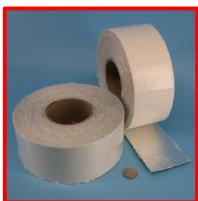
Constructed from a high-temperature base fabric which is then coated with highly-reflective polished aluminum. Designed for long term continuous operation at 650°F / 343°C, this tape will withstand short duration exposure up to 1200°F / 650°C. The aluminum coating melts at 1220°F / 660°C, however it does take some time for the aluminum to absorb enough heat to melt – thereby it can withstand short exposure to the higher temperatures.
