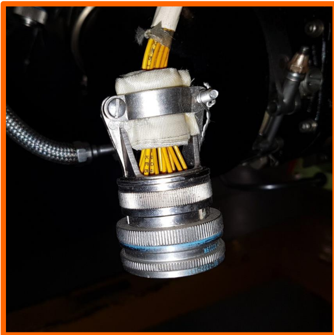
Tape used as a backshell clamp bushing
