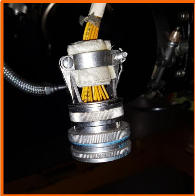
Tape used as a backshell clamp bushing
