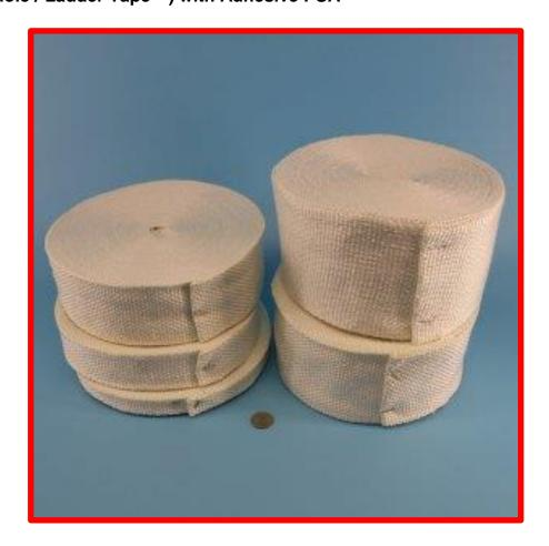
Manufactured of texturized fiberglass yarns, this tape will with stand temperatures up to  $1200^{\circ}F$  /  $648^{\circ}C$  in continuous service. 100% asbestos free, this tape is a bright white color.
