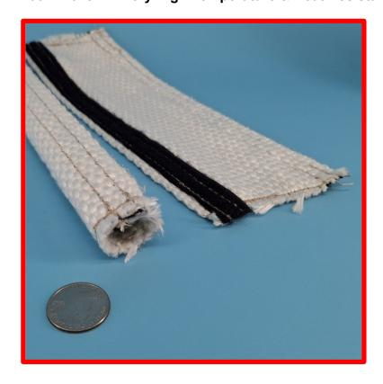
Manufactured of texturized fiberglass yarns, the fiberglass base tape will withstand temperatures up to 1200°F / 648°C in continuous service.
