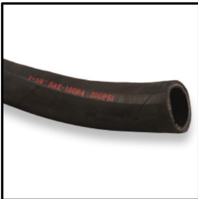
Meets or exceeds SAE 100R4 requirements for low pressure hydraulic return line or suction line for petroleum and water based hydraulic fluids.
