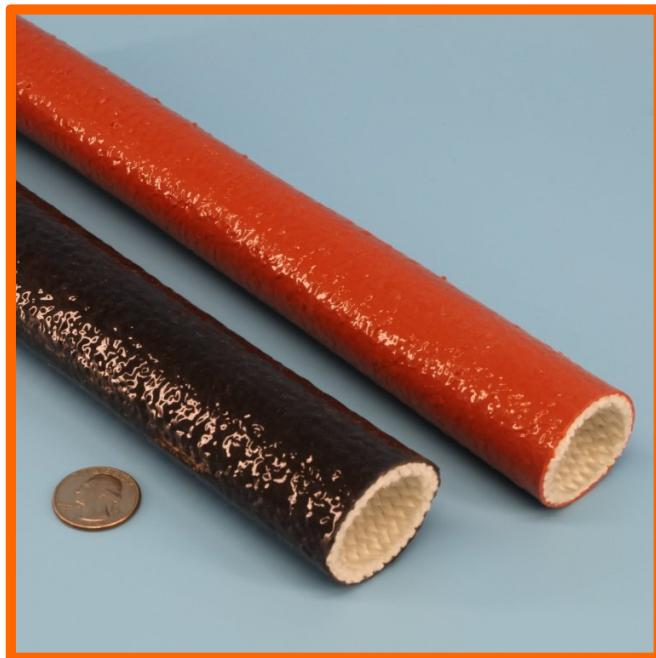
FlameShield™ Aviation / Aerospace grade firesleeve is manufactured to the SAE AS1072F specification and allows properly assembled hose assemblies to meet SAE AS1055D testing. We also maintain traceability records for customers buying this product. 500°F / 260°C rating and with a 15 minute FAA "Fireproof" rating when assembled according to SAE AS1055.
