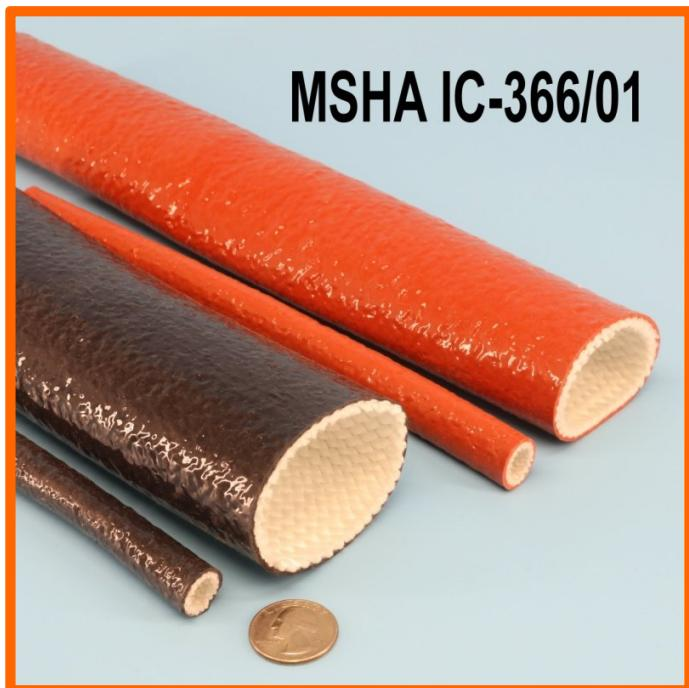
FlameShield™ MSHA Mining approved firesleeve protects hoses and lines on mobile and fixed mining equipment. 500°F / 260°C continuous rating and with a 30 minute 800°F / 426°C rating.
