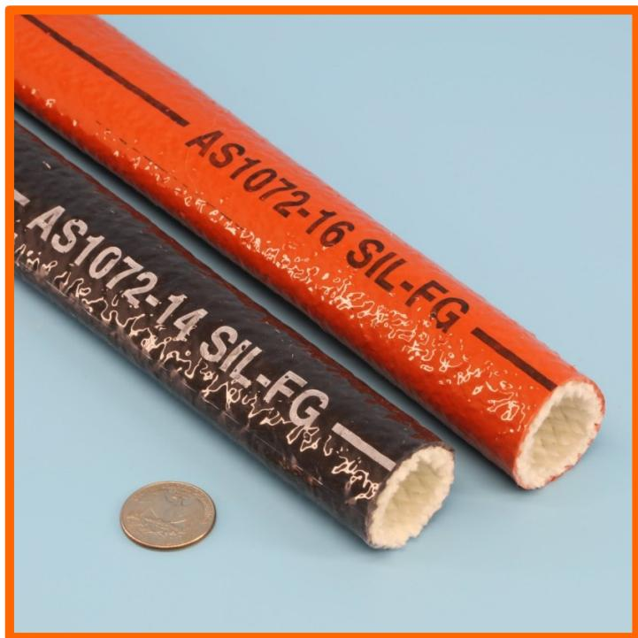
FlameShield™ NSN / NATO firesleeve is manufactured to SAE AS1072 Aerospace specification. CofC and Test Report available with orders. Our company QMS has been reviewed and accepted by major aerospace OEMs. Allows properly assembled hose assemblies to meet SAE AS1055D testing. We also maintain traceability records for customers buying this product. 500°F / 260°C continuous rating and with a 15 minute FAA "Fireproof" rating when assembled according to SAE AS1055.
