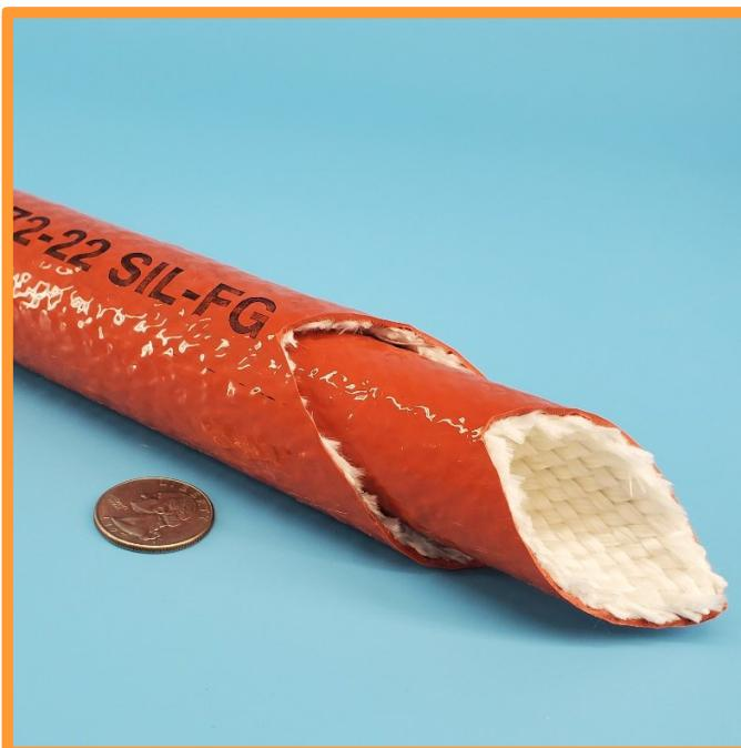
DualShield™ firesleeve is built from two layers of aviation grade sleeve, providing superior protection to hoses, wiring, cables and tubing from heat, flame, molten splatter, sparks and other environmental factors. The first completed sleeve is oversleeved with another layer of fiberglass braid, and that braid is also coated with the same thick coating of self-extinguishing silicone rubber.
